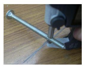
I do not claim this to be a proof, just a demonstration of a possible alternate approach to measuring the pitch diameter. It is certainly easier to handle the split nut than the 3 wires.
