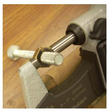
I'm not ready to say that this works but do have some data. The basic idea is to take a hex nut of a given thread size and cut it in half point to point. Deburr the threads and use it to measure pitch diameter. To help get consistent results, I marked one face of the nut so it always goes together the same way.
