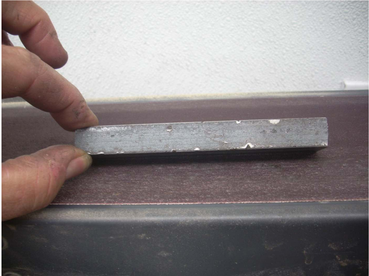
The edges were beveled on my belt sander to remove all burrs.
