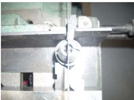
I separated the jaws by using my bandsaw. The surfaces left by the saw blade will be a little rough
