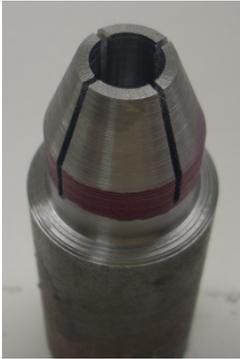
My last machining step was to deburr the saw cuts inside and out.
