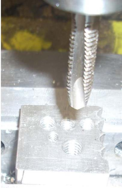
As a test, I have drilled a tap hole and run my 5/16 - 18 tap through it. It performed just as well as my 1/4 - 20 tap held in a real Jacobs Flex collet.
