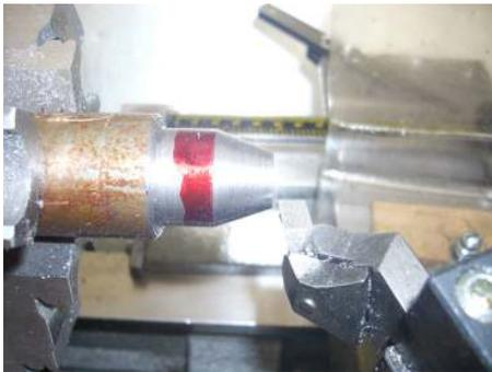
After deburring, I chucked the bar into my lathe and turned the maximum outside diameter for about 1". The collet is about 0.51" long but the excess will not be wasted. It is used to start the next collet.
