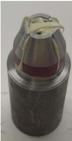
This is the fun part. I squirted 100% silicone caulk into the blind hole and followed by slowly pressing in the shank end of the drill used to make the hole. I then removed the excess from the outside of the part. Inspect each cut to be sure it is completely filled.
