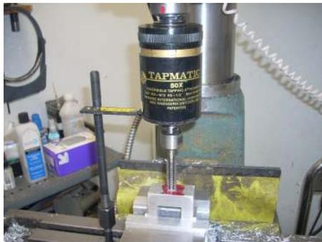
Recently I had the great fortune of receiving a Tapmatic<sup>®</sup> 50X tapping head. It can drive taps as small as a 4-40 and as large as 1/2"-13. To do this, there are a series of Jacobs Flex collets needed. Each one holds a range of tap sizes. For example, the collet that came with the head is good for taps from #4 to 1/4". In
