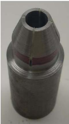
I am left with a neat slab of caulk between each jaw of the collet. The rough saw cuts give the caulk plenty to grab.
