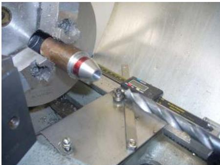
It is then a simple matter of selecting a drill that is close to the diameter of the tap shank I wish to hold. Make your smallest inside diameter collet first for reasons that will become clear soon. The hole is about 3/4" deep.
