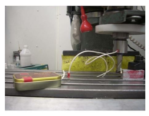
This instrument does not work well on a mill fitted with any common cutter. Mill cutters do not present a single point of contact. Instead, the needed contact point rotates. Only when the spindle is in exactly the right angular position do I get the correct point of contact.
