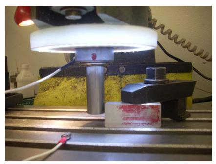
But all is not lost. If I am willing to remove the cutter and substitute a piece of drill rod of known diameter, I get a decent edge finder. A major benefit of this arrangement is that the drill rod is solidly attached to the spindle. No weak, insulating material is in the way.
