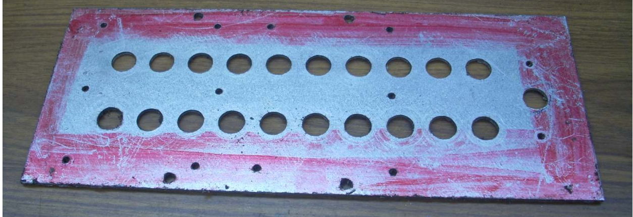
The plate has been machined but not deburred yet. That is red dye and not blood.
