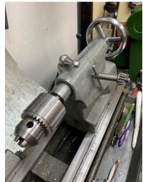
During set up, I can stick the chuck key to the side of my tailstock. When done, it goes back on the shelf.
