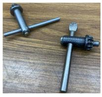
Using Go2 Glue, I stuck a round magnet on the end of each of my chuck keys.
