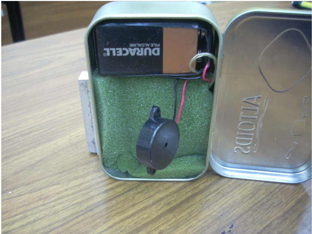
Inside the box is a 9 volt battery and a piezoelectric beeper from Radio Shack ® .
