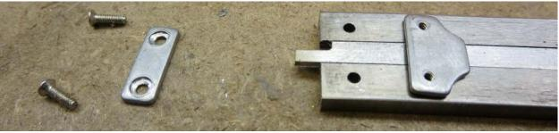
With the two screws removed, the top plate comes off. It is more like a washer and spreads the clamping force over a large area. This is necessary because under that silvery label is an etched strip that is fairly delicate.
