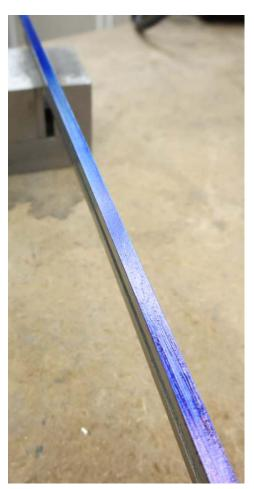
Using Hi-Spot<sup>®</sup>, I coated one edge of the body and placed it down on my surface plate. The resulting variation in blue tells me how far from flat is the edge. I did not see any place where the edge had no blue. So my conclusion is that this edge, on average, is rather close to true. However, it is still rough.
