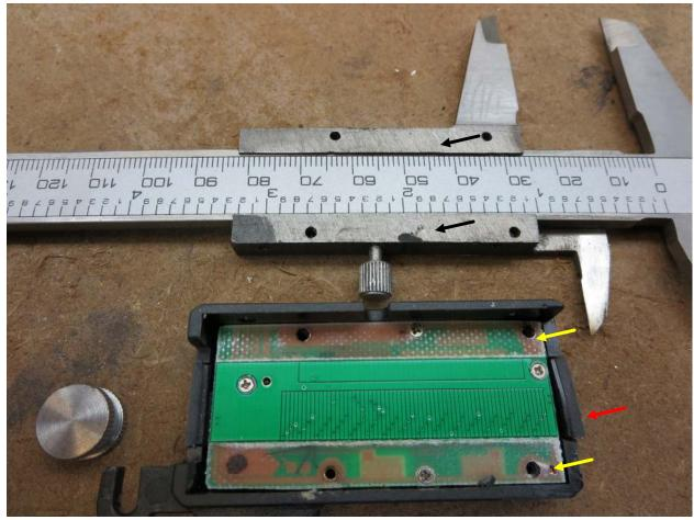
The plastic shell with attached electronics is a snug fit to the metal slider. Hold the slider's body in one hand and pull the shell straight up.
