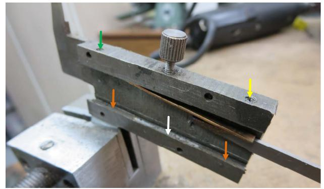
Here you see the bare metal frame of the slider. A phosphor bronze strip attaches to the top side. (Poorly) machined reference surfaces (orange arrows) can be seen at the bottom. Between these surfaces the metal is roughly cut away so it does not contact the edge of the body (white arrow).
