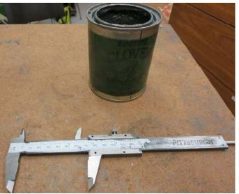
As a final smoothing operation, I used some Clovis<sup>®</sup> 500 grit lapping compound on the body and slider.
