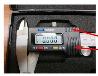
The installed battery was still good so after pressing the OFF/ON button and then the inch/mm button, I saw inches on the display.
