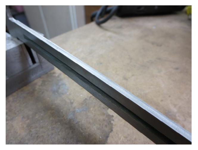
This is a close up view of the edge of the body. Notice the cross grind marks. As the slider moves along this edge, it must ride over these marks. This is the main reason for the rough feel of the instrument. It sounds and feels a bit like dragging a rake across a slab of concrete. Fortunately, this surface finish can be improved using commonly found tools. This does require disassembly of the caliper.
