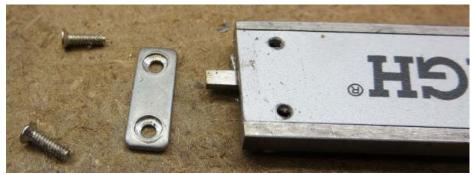
Before trying to remove the slider, the clamp on the end of the body must be disassembled.
