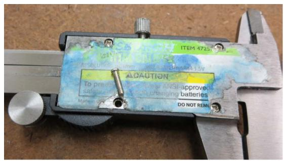
The three screws that cut into the plastic have been installed and I'm about to install the one bolt.
