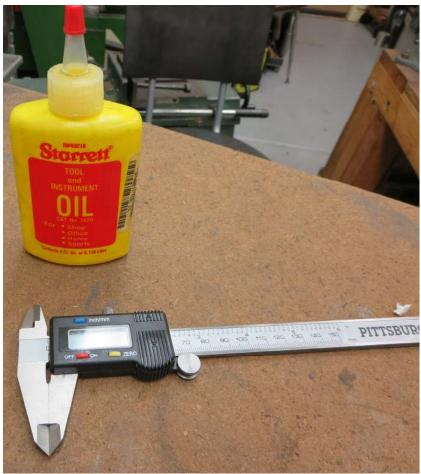
As a final step, I used a very tiny amount of instrument oil on all sliding surfaces. One or two drops is plenty. When done, wipe the caliper down with a clean/dry cloth to remove excess oil.
