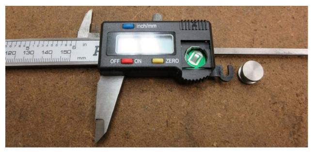
I pressed the plastic case down on the metal slider body and then moved the slider to the end of the body. It is then possible to install the thumb wheel.
