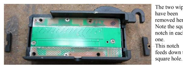
The two wipers have been removed here. Note the square notch in each one. This notch feeds down the
