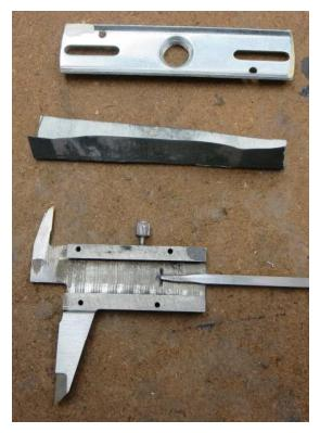
My first task was to smooth the inside of the slider. I used a piece of steel with a lip bent into it and some fine emery cloth.
