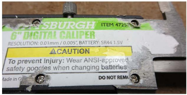
Oh well, not as nice now. Digging around I have uncovered the four screws that hold the body together. Once apart, you can soak the rest of this label off.
