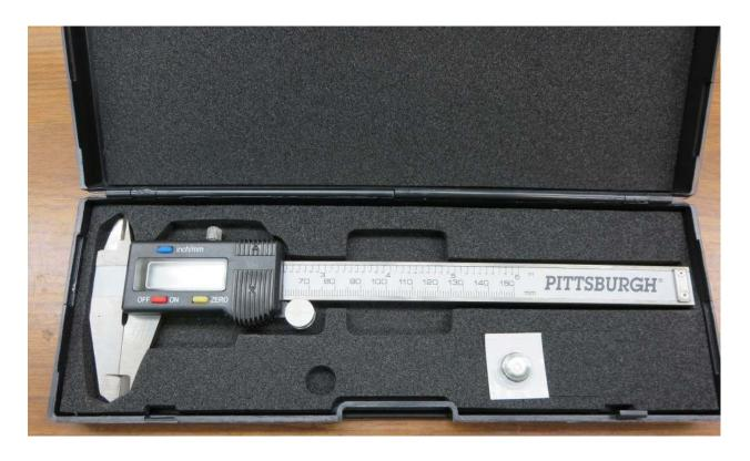
When the shrink wrap is removed and the cardboard sleeve discarded, are able to open the lid on the case. The caliper you find has one battery already installed plus a spare. I have often found the installed battery to be dead so the extra one is appreciated. These batteries are alkaline and have a much shorter life than the silver oxide variety.
