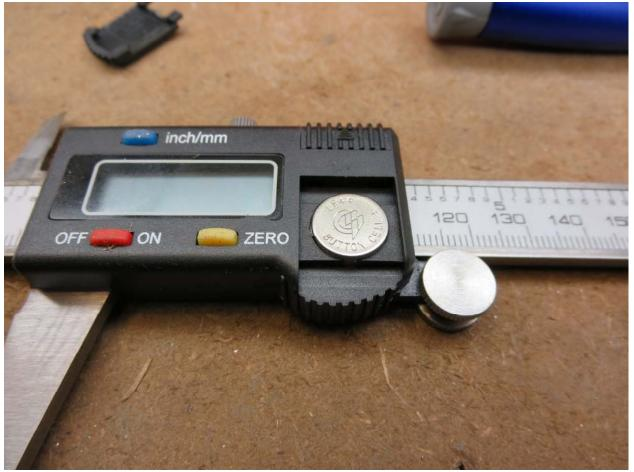
Remove the battery before performing further disassembly. We don't want to short anything out and blow the circuit.
