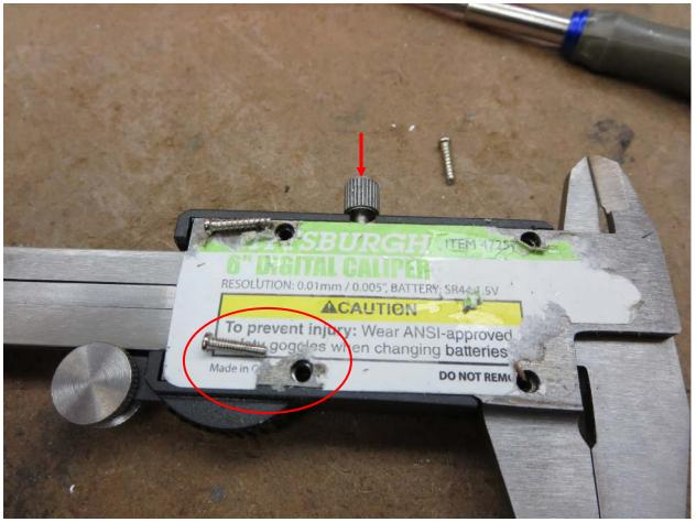
Using a small Phillips head screwdriver, I removed the bolt in the lower left corner. This bolt threads into a bit of metal which secures the thumb wheel support.
