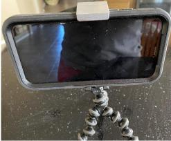
This time the prototype worked well. The adapter reached over the top of the phone while the arm was partially extended. The top lip held securely without blocking any of the screen.
