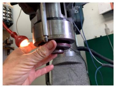
What a perfect storm. The spindle-bearing grease cup screws in upside-down and has fine threads on its perimeter. It is also greasy, making it hard to hold and turn.
