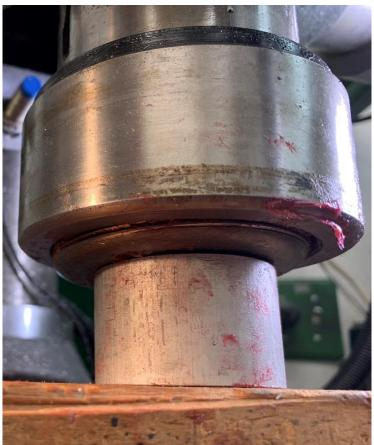
Then I slowly fed the Z axis down until the cup was inside the end of the spindle. The trick was to get the threads close enough that I only had to turn the cup to engage the threads.
