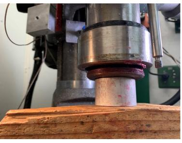
After the usual false starts, I selected a short length of aluminum thick-walled tubing. It cleared the spindle while supporting the cup.
