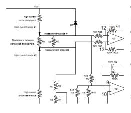
There are a few loose ends here.  $R_2$  and  $D_1$  can be found near  $R_x$ . They do nothing under normal circuit operation. When the measurement probes are removed from  $R_x$ , their voltages would be undefined and that can lead to strange behavior or even damage to the op amps. So instead I have  $R_2$  which ties the measurement probes together. The 1K value has a minimal effect on the value of  $R_x$  seen by the rest of the circuit.
