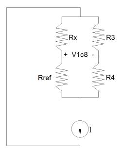
At the heart of the circuit is a Wheatstone bridge. A constant current source, marked "I", feeds the circuit.
