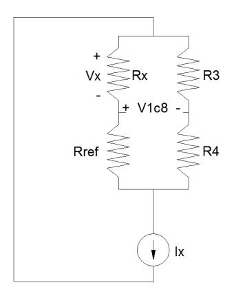
Recall that the current that flows through my Wheatstone bridge comes from a Voltage Controlled Current Source. It is defined by equation 1:
