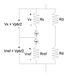
Going back to the high level schematic, I have added in my high current probe #2 voltage drop,  $V_{pb}$ . Thanks to R3 and R4, this unknown voltage has been equally shared by  $V_x$  and  $V_{ref}$ . Balance is detected when
