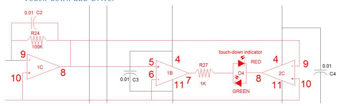
The output of op amp 1C with respect to  $V_{1C10}$  drives a pair of op amps used as comparators. When this voltage is positive,  $V_{1B7}$  swings up to near the positive power rail while  $V_{2C8}$  swings to near the negative power rail. This causes current to flow through the red LED. When this voltage is negative, the green LED lights. If this voltage is very close to zero and there is any AC noise, both LEDs will dimly light.
