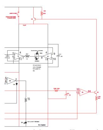
This current is drawn from the parallel combination of  $R_{29}$  and the base of  $Q_4$ . Since  $V_{be4}$  is around 0.7V, this leaves
