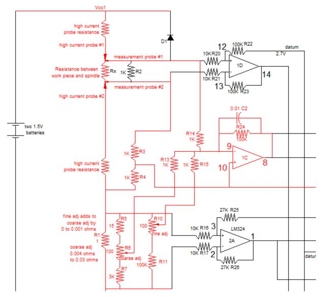
Starting at the top, I have the battery voltage which is marked  $V_{cc1}$ . It is around 2 volts when my test current is 1 amp. Those 1.5V batteries drop a lot of voltage with this kind of load.
