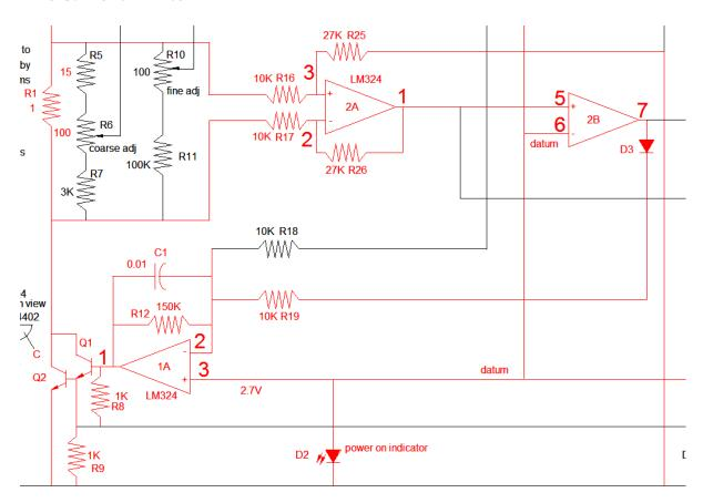
The current through  $R_x$  must not get above 1 amp. This function is accomplished by directly measuring the voltage across  $R_1$ . This voltage equals our test current times  $R_1$ . So at 1 amp, op amp 2A sees 1V. It amplifies this voltage by 2.7 to generate the voltage  $V_{2A1}$  which is with respect to my negative power rail. Op amp 2B is used as a comparator. It compares  $V_{2A1}$  to the voltage across  $D_2$  which is about 2.7V. I get a state change in 2B when
