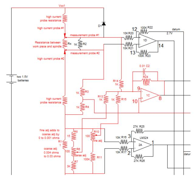
My goal is to compare the voltage across  $R_x$  with the voltage across my  $R_{ref}$ . The problem is that I have an unknown voltage drop in the "high current probe #2" between them. I don't know what this voltage drop is but I sure can divide it in half with R3 and R4. Doing this gives half of this unknown voltage to my  $R_x$  voltage drop and the other half to my  $R_{ref}$  voltage drop.
