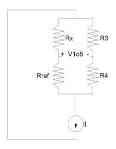
In a regular Wheatstone bridge I adjust  $R_{ref}$  to be equal to  $R_x$ . But  $R_x$  is in the milliohms and I don't have a potentiometer in that range. Not to worry, what I really want is the voltage across  $R_{ref}$ . I don't care about the value of  $R_{ref}$ , just the voltage.
