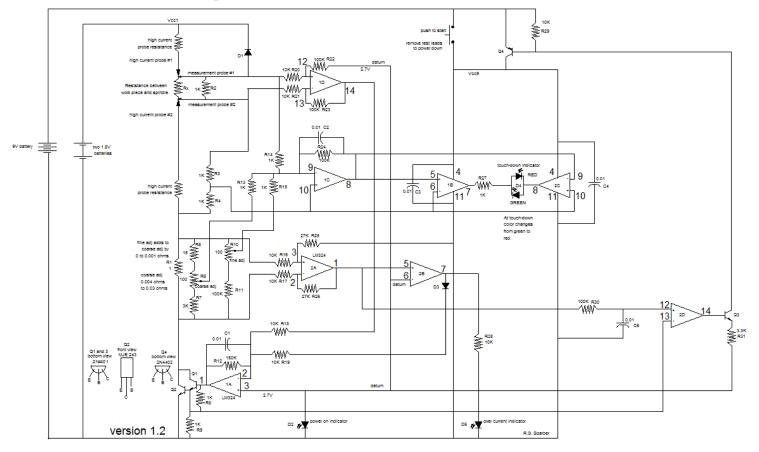
The circuit uses two quad op amp ICs, one power NPN, a few small signal transistors and diodes, and a bunch of resistors and capacitors. It is powered by a 9V battery and two 1.5V batteries.
