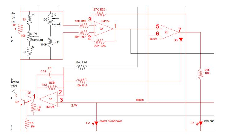
This turns on diode  $D_3$  and applies about 7V to  $R_{19}$ . This large flow of current into amplifier 1A cause  $V_{1A1}$  to slam down to near the negative power rail. Q1 and Q2 quickly turn off so no current flows through  $R_1$ .
