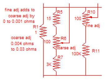
So instead of having an Rref of, say 10 milliohms, I have R1 equal to 1 ohm. Then I use a voltage divider to cut this voltage down to the level I would get if my test current passed through a 10 milliohm resistor.
