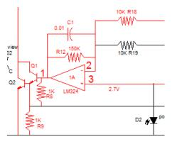
But since current is flowing through  $R_x$  in order to generate  $V_x$ , I know that  $Q_1$  and  $Q_2$  are on. Therefore, the voltage at pin 1 of op amp 1A must equal  $V_{be1}$  +  $V_{be2}$ .
