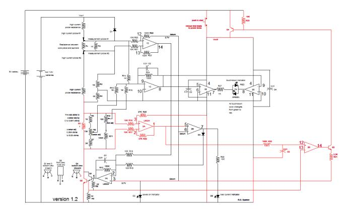
When the test current falls below about 0.25 amps, the circuit powers down. In this way, when you remove the test probes, you can't leave the power on to drain the batteries.
