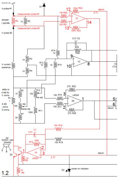
Op amp 1D directly measures the voltage across  $R_x$  and multiplies it by 10. But wait, wasn't my ground pin 10 at op amp 1D? Well, I lied a little. While true for op amp 1C, I use a different "ground" for op amp 1D. I will call it my "datum". All this means is that my voltage V<sub>1D14</sub> is with respect to my datum. I did this to move my output voltage of op amp 1D away from the negative rail of the power supply. It also has another use which will become evident soon.
