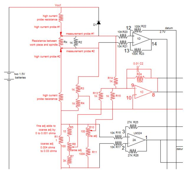
One nice thing about using an op amp to measure my effective  $R_{ref}$  is that I can simply add the fine adjust current to the coarse adjust current to get the full effect. So I can set my coarse adjust pot to 10 milliohms and use the fine adjust to move the effective  $R_{ref}$  between 10 milliohms and 11 milliohms.
