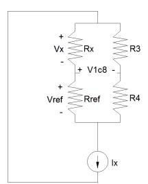
The circuitry in red may not look like a Wheatstone Bridge but it follows the same logic. R14 in the schematic corresponds to R3 in the simplified diagram. R1, R5, 6, 7, 10, 11, 13, and 15 are represented by R4 in the simplified diagram. And the voltage out of op amp 1C, pin 8 is my  $V_{1c8}$ .
