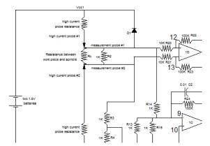
The input transistors in these op amps are PNPs so current flows out of them.  $D_1$  provides a path for this current into the two 1.5V batteries. I used a diode here rather than a resistor because I do not want any current to flow from these batteries into the rest of the circuit when the probes are removed.
