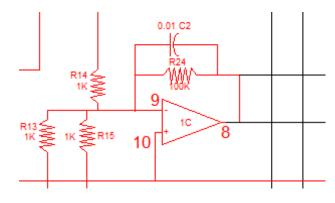
Capacitor  $C_2$  causes the op amp to have less gain as the incoming signal increases in frequency. Since the only signal I care about is at DC, this cap is helping reduce any unwanted signals.  $C_2$  with  $R_{24}$  create a corner frequency of 318 Hz.
