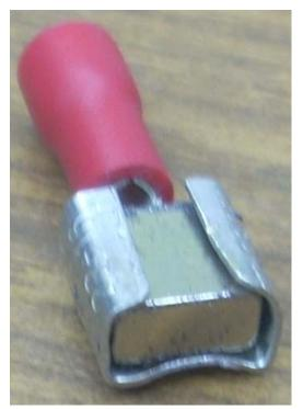
Then use a pliers to form the sides around the magnet. Bend up the front a little so it doesn't fall out. The clip is now ready to have a wire put in the other end and crimped.
