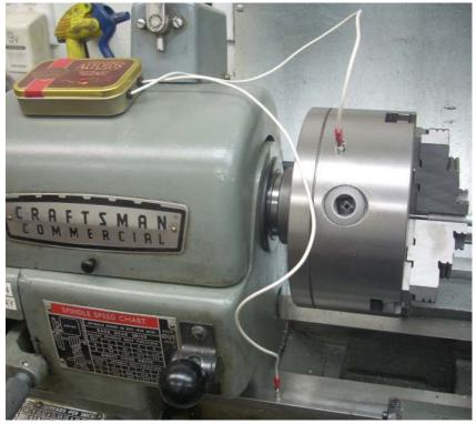
Here you see the clips in action. It would be impossible to make these connections with alligator clips. But with the magnetic clips, I just toss them onto the surface. And as an added bonus, any oil left on the surfaces is pushed aside by the strong force of the magnets.
