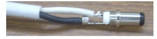
I slid on a piece of white heat shrink tubing before attaching the wires to the male connector.
