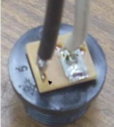
Here you see the white wire soldered to the central pin of the female connector. The black wire connects to the outside contact. I trimmed off the excess tab on the central pin connection.
