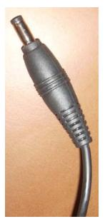
The power plug has a massive strain relief on it. This strain relief protects the low cost power cable from pulling out of the low cost plug.
