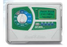
My irrigation controller operates 6 zones. This requires one wire per zone plus a common return wire. At the present time I have a 7 wire cable so there is no room for growth. This cable is under a slab of concrete so replacing it is not an attractive option. When the controller applies about 24 volts AC to a valve, it opens.
