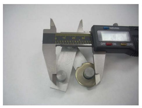
Next I slip a thick washer over the post attached to the rear blade. This helps me align my digital caliper squarely on the sides of the posts. I record the reading.
