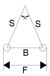
I have measured the diameter of one post. Since they were all cut from the same rod, they *should* both be the same diameter. If they are not, you can turn them to the same diameter or change to drill rod. You could also just live with the error by carrying the radius of each post in the equation. Now, if the posts are not round, then replace them.
