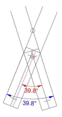
Next, consider the case of one blade not having its holes on its center line. The angle formed by the line connecting the center of the left post with the pivot is the start of the angle. The center line of the right blade is the end of the angle. I read 39.8°.
