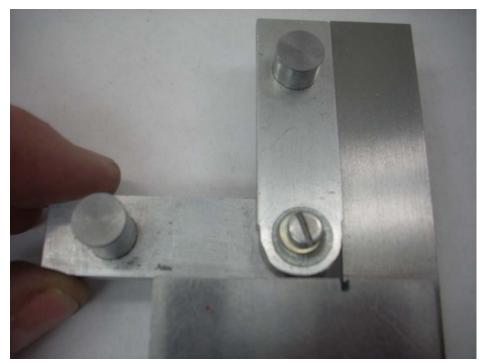
Here I am calibrating the gage with my 2" machinist square. Once the angle has been set to 90°, I lock the pivot.
