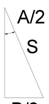
If I drop a line straight down from the top of this triangle to the base, I get a right triangle with hypotenuse, S, and an angle  $\frac{A}{2}$ . The base has a length of  $\frac{B}{2}$ .
