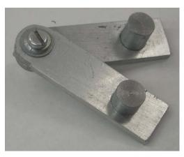
You will need to cut off a 0.25" length of 3/8" CRS rod, face the ends for an overall length of about 0.24" and drill a clearance hole for a 6-32 screw. That is the pivot. If the rod is not round enough, you could use drill rod.
