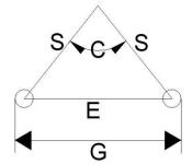
All parameters in red are known. So what is left is a way to translate the desired angle, C, into a distance between posts of G
