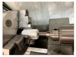
Going to my lathe, I first cut a bevel in each end. Then I drilled a ¼ inch hole in each end to a depth of 0.9 inches. This was necessary to meet the required overall length.
