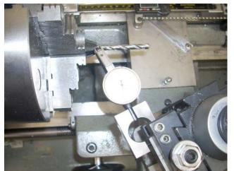
You are looking down on a lathe set up. On the left is my 3 jaw chuck. Held in the chuck is a drill being used as a mandrel. On the drill shank is a Jacobs Flex collet. Contacting the Flex collet is my Dial Test Indicator (DTI) which is clamped to a support that is fixed to my Quick Change Tool Post.
