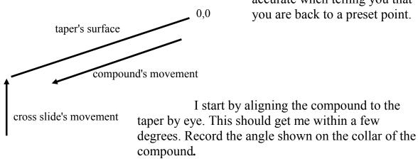
Then I feed in on the compound and the cross slide until I read 0 on the DTI at the 0,0 point shown above. All subsequent readings of the dials are done by feeding in so as to avoid backlash error on the lead screws.
