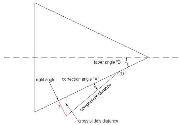
Our goal is to adjust the compound's angle to match the taper angle. I have a fairly good idea what the taper's angle, B, is because I have adjusted the compound by eye to get close. The estimated taper angle equals 90° minus the compound angle.
