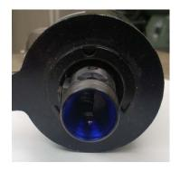
Here is the female taper that will receive the taper I will make. The inside surface has been lightly coated with Hi-Spot ink and will remain wet for a long time.
