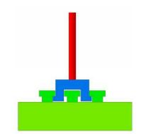
Here is an end view of a C-nut engaged into a pair of T-slots. The C-nut is blue, the stud is red, and T-slots are green. The C-nut straddles what I call an island formed by two T-slots.
