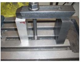
Here is a typical application of a T-nut, threaded stud, support block, clamping bar, and hex nut. The closer the stud is to the part being clamped, the larger percentage of the force is applied to it.
