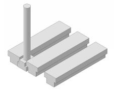
When used for clamping, there is an upward force that lifts the T-nut until it makes contact with the underside of the lips.
