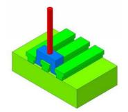
The upward force passing through the stud lifts the ears of the C-nut and applies pressure to the lips of the T-slot. Ideally, the forces are identical to a T-nut. In practice there will be some bending of the C-nut so the ears are expected to bend slightly. This will put more force on the ends of the lips. I plan to run a test to see if this is a problem.
