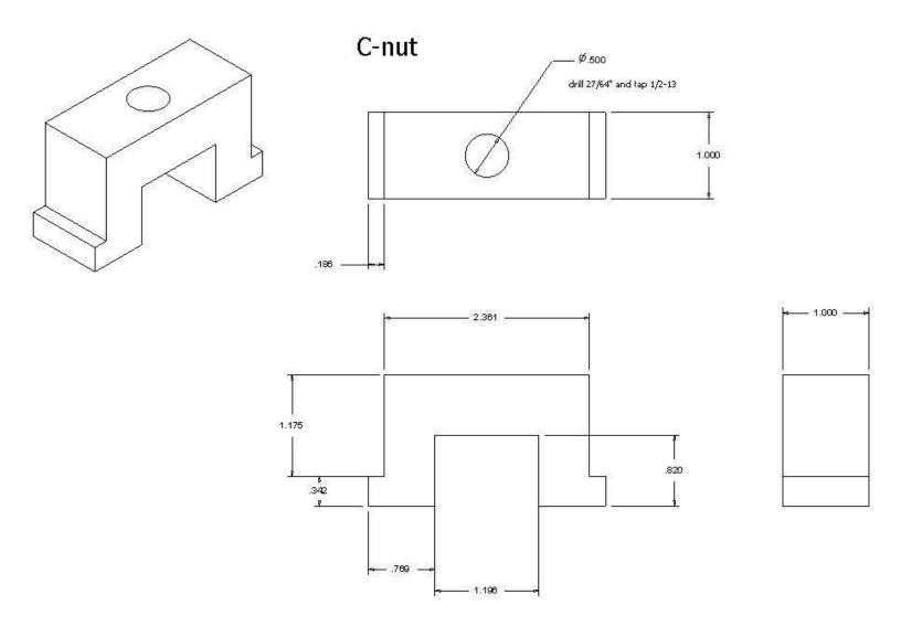
I will adjust the 1.175" dimension to fit the stock I have on hand.
