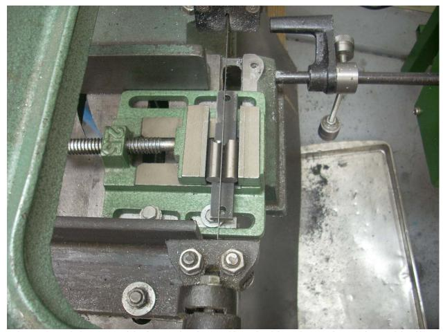
I then placed the assembly in my horizontal/vertical bandsaw vise so it could still slide side to side. With the saw off, I lowered the blade into the gap between rods. With a little wiggling, I could feel it drop in.
