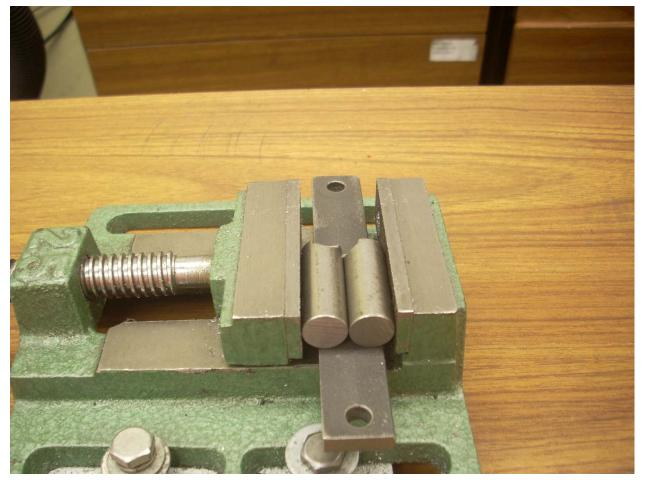
I started by clamping two pieces of ½" round stock in the vise. The bar was necessary to prevent the right bar from falling in the gap between vise ways and fixed jaw.
