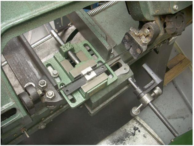
To test my alignment, I put a block of aluminum in the vise and made a cut about 0.1" deep.
