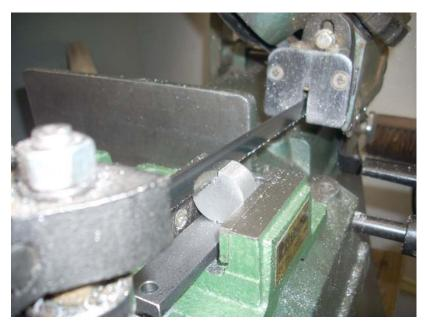
Recently I needed to cut a cylinder longitudinally along its diameter on my horizontal/vertical bandsaw. The cut was not critical but I did want it to look good. I was off by maybe 0.02" which was serviceable but certainly not pleasing to the eye. That got me thinking, how can I better align my blade for a closer cut. Here is how I did it.
