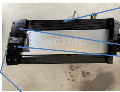
I ripped a 2 by 4 to be the same width as the battery's thickness and cut two lengths. These flank the battery.
