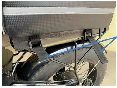
The side straps pass under the rear rack and into square loops. By folding the straps back under the rack, the trunk is secured.
