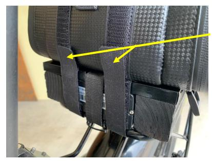
The front straps pass between the battery and the rear rack, loop underneath, and fold back onto the trunk. Velcro secures them. A quick tug on these straps releases the trunk.
