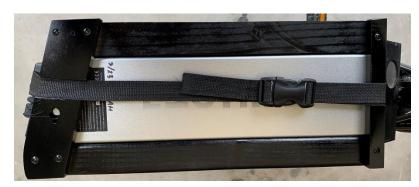
The strap in the two recesses prevents the battery from moving forward and back.
