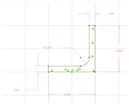
I have finished defining my cross section using the dimension tool. I also moved the radius label so it is more readable. Just drag it around to place it.
