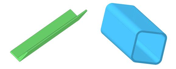
This is how I draw angle iron and square tubing using the Computer Aided Design program called Alibre PE. The key tool to use is the *extrusion* function. I draw the cross section and extrude to the needed length (the tool calls it depth).
