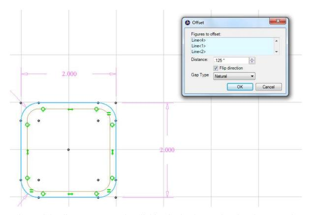
I changed the distance to .125" by clicking in that box and typing the new value. I then checked the Flip direction box and then things look right. Note that the tool changed the inside radii in order to keep a constant distance of .125". My cross section was then done.
