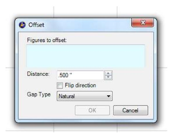
Up came the Offset dialog box. I must select which lines I want to copy and offset plus specify the Distance to offset if I don't want the default of .500".
