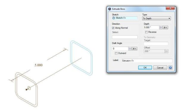
As with the angle iron, I called up the Extrude Boss tool. In this case I have decided to accept the Depth of 5.000".
