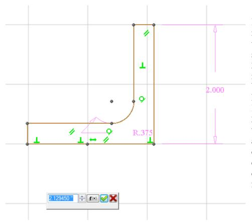
I clicked on the right most vertical line and set its length to 2". Here you see me setting the bottom horizontal line length. It was at 2.129450" and I will just type 2 and hit enter. The data entry box's default is to directly accept a number.
