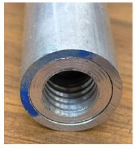
Here is one example. I have thin-walled aluminum tubing with an inside diameter of  $\frac{1}{2}$ ". I want to screw in a 3/8-16 bolt. My homemade anchor solves the problem.
