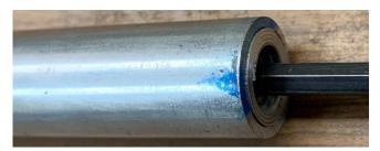
I have found that the lock digs in well enough that I do not need to grab the body as I tighten the SHCS. This lets me set the anchor flush with the end of the tubing.
