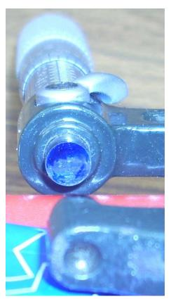
It got me thinking. Although not as sensitive, I can use some Dykem Hi-Spot on the anvil and see how much prints onto the spindle. Clearly I have found another error source. I don't yet know how much error it contributes but by mic'ing on the blued area and then on the clear area, I should be able to tell.
