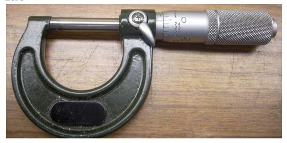
After carefully cleaning of the anvil (the fixed part), and spindle (the movable part) of the mic, we gently turn the thimble until the anvil touches the spindle. The thimble should then read exactly 0. In my case it does. This is necessary but not sufficient.
