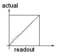
In this picture we have a red dashed line that represents perfection. The blue line is reality. Note that there is a range of values that are wrong. Yet the rest of the mic's travel is close to perfect. This kind of error implies damage to some of the threads on the rod.
