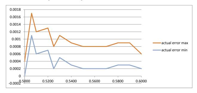
Note from the above tests that when I measured my 0.5000" spacer block for the Linearity Test, I got 0.5003" +/-0.0002" but when I did it for my Threaded Sleeve Test I got 0.50002" +/-0.0002". They are within the uncertainty limits. Similarly, when I read 0.6000" for the linearity test, I got 0.6001" +/-0.0002" yet for the Threaded Sleeve Test I got 0.6004 +/-0.0002". This too is within the uncertainty limits.
