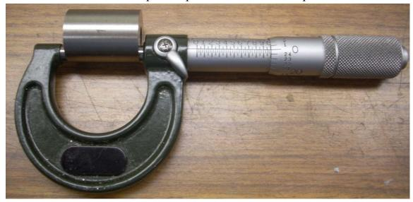
The thimble should then read exactly 1.000". In my case it does. This too is necessary but not sufficient.
