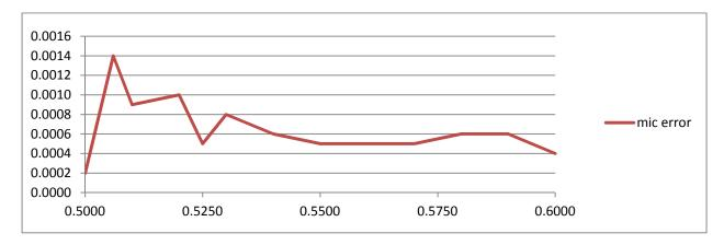
The horizontal axis has a tick mark at each place that the thimble reads 0. Note that the graph has a local minimum at each of them. This implies but does not prove that errors in the threaded sleeve are the cause of this error. However, it does illustrate that we do have a lot more error than might be assumed by just looking at a few points.
