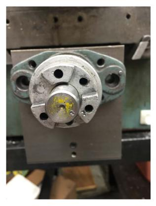
If you are trying to reduce the backlash on the Y axis, your first step must be to align the leadscrew to the ways. Only then can you tighten up the nut and not have binding. The problem is that a very small shim under one side of the bearing flange causes a rather large swing in the lead screw's alignment. The ratio is about 12 to 1 and you really want to be aligned to within about a thou.
