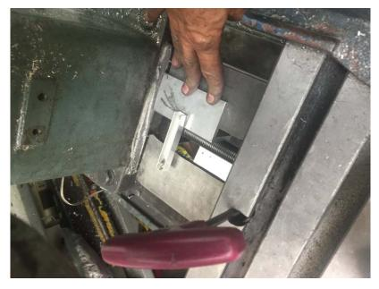
When you are satisfied that the Y leadscrew is aligned correctly as viewed from the top, the final step is to lock its position. This is done by firmly holding the thick angle with one hand and tightening the nut with the other. Do a final check of alignment before moving on.
