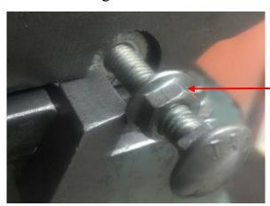
One source of drag is a Y ways gib that is able to slide as the apron moves in and out. I solved this problem with an improved Gib retainer. see <a href="http://rick.sparber.org/GR.pdf">http://rick.sparber.org/GR.pdf</a>
