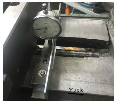
The instrument is now in the zero set position. The pushrod of the DTI is about 1 inch from the center of the take up nut's bolt. This distance is our "A" value to be used in equation (8).
