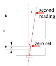
Using a steel ruler, measure the distance from the center of the take up nut's bolt to the zero set point of the DTI. Call this distance "A". Distance "B" is from bolt to the second reading location.
