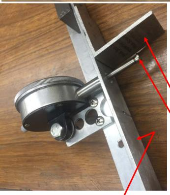
I'm using a second push rod DTI. Since it is necessary to switch between measuring yaw and roll, it is far more convenient to have two DTIs. The block of steel bolted to the angle prevents the instrument from tipping over.
