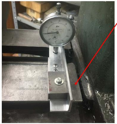
Note that I'm not actually contacting the ways which are at the bottom of the dovetails, but rather this surface above the ways. Measurements say it is good enough.
