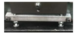
Using a wrench, the two vertical jack screws raise the plate while the leadscrew tilt is monitored. This monitoring requires another measuring instrument.
