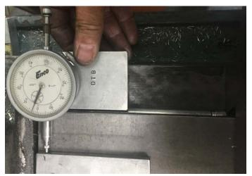
If the DTI needle moves, my yaw is not zero. Here you see an error of 0.003 inches. That must be brought down under 0.0005 inches.
