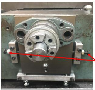
Here you see the bearing block and leadscrew installed on the pins. Bolts will be added later to clamp the bearing block to the plate and to the mill's base. The bearing block must be snug against the plate. To begin with, this is accomplished by turning the leadscrew such that it pulls in. Later bolts are added.
