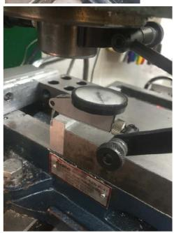
I then moved the table along the Y axis a distance of 3 inches and did not see any binding. The backlash increased to 0.0020 inches.
