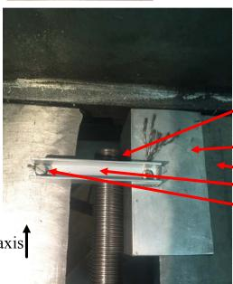
With the apron moved forward, a gap is reveled with the Y leadscrew inside.
