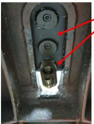
Looking from under the mill, you can see the the bottom of the apron and the take up nut. The Y leadscrew has been removed.
