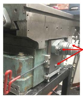
By adjusting the horizontal jack screws I can smoothly swing the leadscrew until the yaw is zero.
