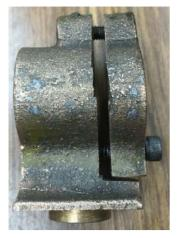
As manufactured, the take up nut tends to push the leadscrew's major axis out of radial alignment with the nut's major axis as backlash is removed. This can be solved by modifying the take up nut. See <a href="http://rick.sparber.org/YTUN.pdf">http://rick.sparber.org/YTUN.pdf</a> for details.
