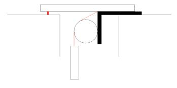
The string is run over the top of the leadscrew and the weights hang down. The string then pulls the angle tightly against the outside diameter of the leadscrew and also down against the right top surface. The horizontal channel bar prevents the angle from rotating. The screw (shown as a red
