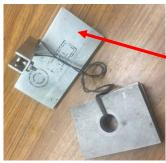
This odd collection of scrap from my junk drawer is actually half of a precision instrument for measuring yaw. There is a piece of extruded 2 x 2 inch aluminum angle about ¼ inch thick. It attaches to a short piece of U channel that has an adjustable screw on the end. Looped around this channel at the angle end is a string. The string connects to a series of weights.
