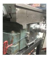
Recall that this alignment is done by loosening one horizontal jack and tightening the other.
