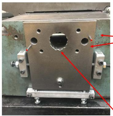
As manufactured, it is impossible to change the alignment of the Y leadscrew. My solution was to create a new mounting support. It can be positioned independent of the base casting.
