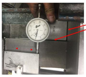
Here is the entire assembly. The DTI contacts the angle's vertical edge nearest the front of the mill. The DTB block contacts the back of the apron. Since the left edge of the DTB block contacts the rod contacting the ways, movement of the block and therefore the DTI is parallel to the ways.
