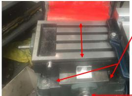
As the leadscrew turns, it drives the apron in and out. The path taken by the apron is set by its ways.
