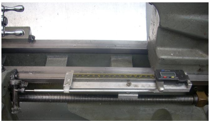
Here you see the entire attachment. It consists of a digital caliper that has been modified and clamped to a plate of aluminum. A steel rod links the slider of the caliper to a screw that can be seen on the left. The right end of this rod was heated and flattened in order to make bolting it to the slider easier. Under the center of the plate is a clamp that secures the attachment to the ways. The rod is supported by a cable clamp on the left so it does not flop around when not in use.
