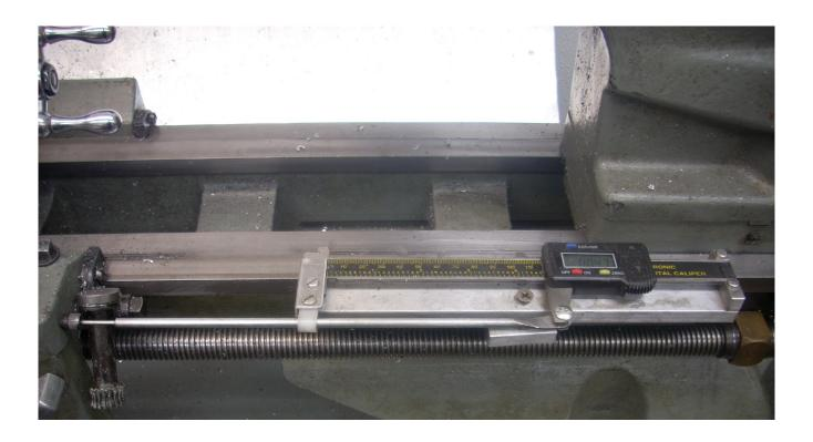
With the way clamp and screw tight, movement of the apron is measured by the caliper. Note that the left end of the caliper is clamped down to its support block. The right support block permits the caliper body to slide back and forth due to thermal expansion but not lift out. This arrangement prevents stresses from building up in the caliper's body.
