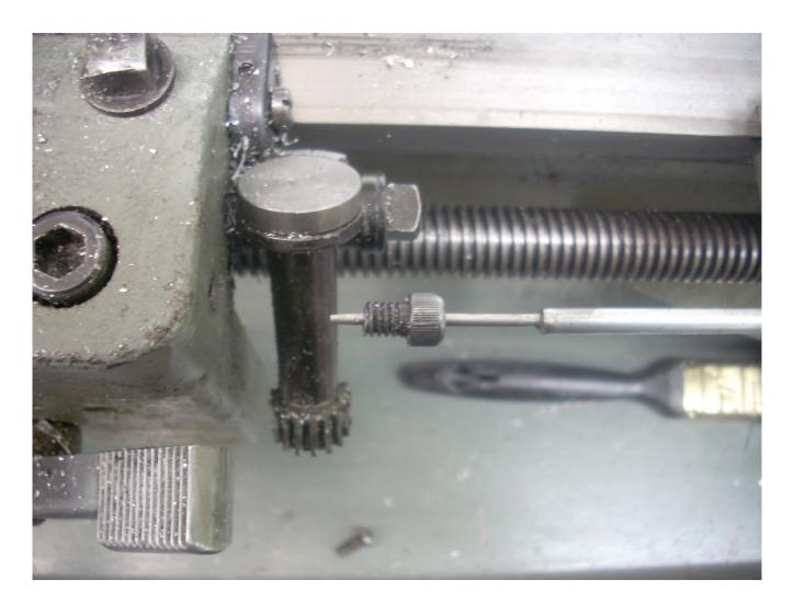
Here is a close up of the screw. It is just a cap screw drilled out and slid over the stiff wire. Fortunately, the center of the screw was soft.
