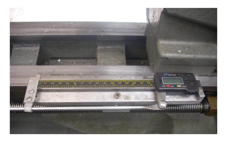
The caliper is made from stainless steel of unknown hardness. I drilled one of them easily with a HSS drill bit. The next one I tried to drill was barely scratched by such a drill. Recently I needed to drill another one and found that a new 3/16" carbide tipped concrete drill worked very well.
