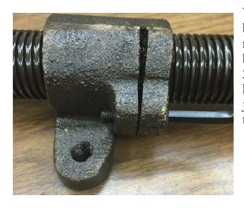
With the leadscrew assembly on your bench, it is easy to access the take up nut. I tightened mine almost to the limit because there was so much wear from 25 years of use. I also didn't want to have to pull this assembly out again just to snug up this screw one more time.
