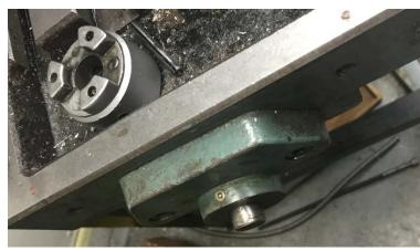
Remove the spline hub from the left end of the table by driving out the roll pin. The same suggestion stands: make marks in both the hub and shaft before removing anything.
