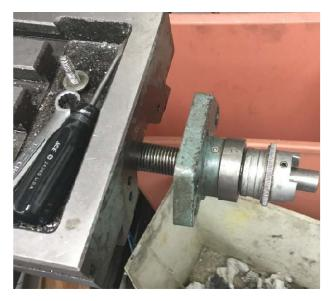
Remove the two screws from the right side bearing flange. You should then be able to pull the leadscrew assembly out.
