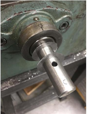
The spline hub has a recess on the back side. At the bottom of the recess is the contact area for the bearing. It is not possible to directly insert a feeler gage to measure the needed shim thickness. Although I didn't do it, the smart approach here would have been to measure the movement of the shaft before the hub was removed. Then use a shim to equal this play.
