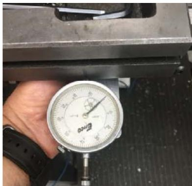
Then it is moved to near the right bearing. In this case I read zero so the leadscrew is aligned to its ways in the XY plane. Yaw is now zero.
