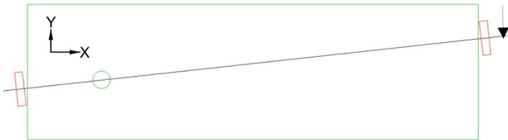
In this top view, you see that the right bearing is crazy far out of alignment with the left bearing. We need to push it forward. This will rotate the leadscrew clockwise on the XY plane. Recall that this motion around the Z axis is yaw.
