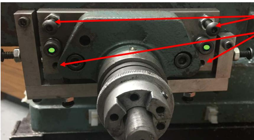
Two top screws plus two bottom set screws carry the force of the two mounting bolts (under the green dots). In this way, the mounting plate can be tilted as needed to follow the leadscrew.
