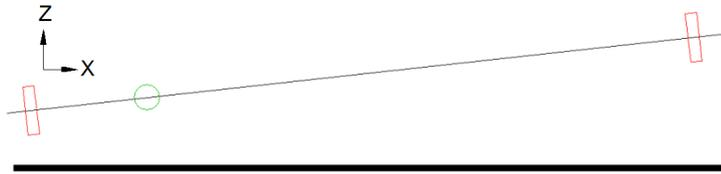
The thick black line is the ways. The two red rectangles are the bearings and the green circle is the take up nut. The right bearing is higher than the left.
