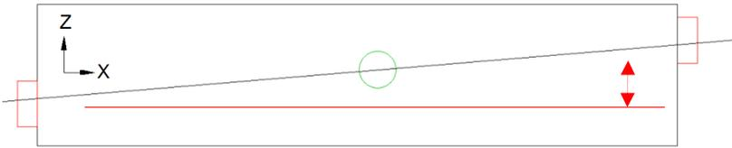
This instrument can tell us when we have zero pitch. When pitch is zero, the leadscrew is parallel to the XY plane.
