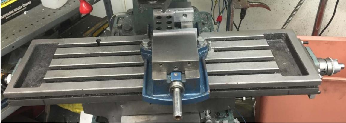
The RF-30 Mill/Drill uses a leadscrew and take up nut to move the table along the X axis (left/right movement). When converted to Computer Numerical Control, minimizing backlash in the leadscrew/nut arrangement becomes critical. It must also change as little as possible as the table moves. This is because the CNC software can cancel a fixed backlash but any deviation will become positional error.
