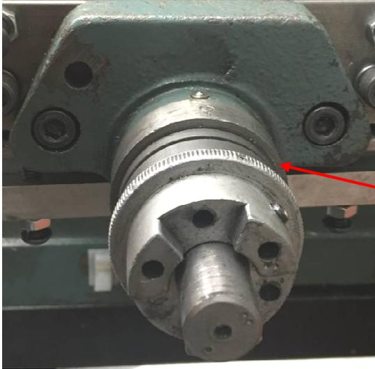
Inside the right bearing block are ball bearings that are intended to permit easy rotation of the leadscrew while preventing movement along the X axis. As manufactured, the leadscrew was able to slide in and out about 0.01 inches. The addition of a variable thickness washer let me preload the bearings and remove all but about 0.0001 inches of axial motion. This axial motion directly adds to my X axis backlash. See <http://rick.sparber.org/VTW.pdf> for details.
