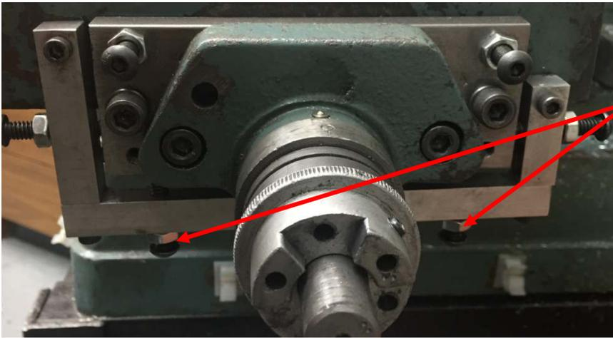
Jack screws on the bottom enable us to perform this motion.
