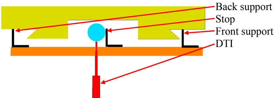
With the instrument in place near the left bearing, the DTI is zeroed.
