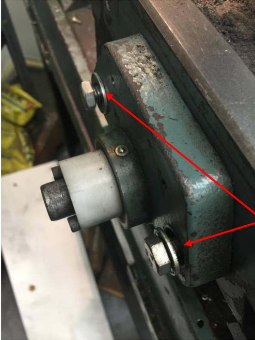
The take up nut is first tightly bolted to the apron and the leadscrew fed through until it enters the left bearing. This is loosely attached to the table. The right bearing is then loosely fitted.
