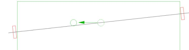
This is the same as saying that the nut moves to the left with respect to the table. Due to the misalignment, the nut will see both this rotation and a movement perpendicular to the table motion. When the leadscrew hits the inside of the nut and the threads bottom out, table movement stops.
