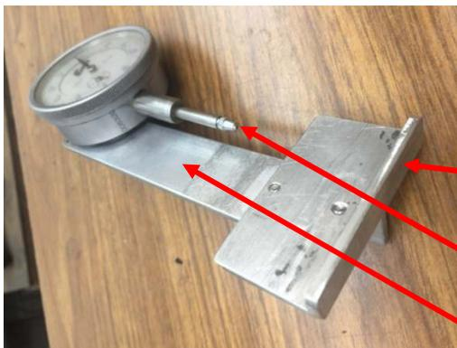
The cut down angle part contacts the leadscrew and the DTI contacts the dovetail.
