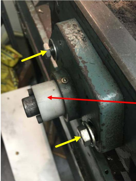
The left bearing support was badly worn after 25 years of half hearted lubrication. I saw about 0.02 inches of play between "bearing" and leadscrew shaft. This bearing was just a hole through the casting. Since I'm trying to align the leadscrew to within 0.0005 inches over its length, I cannot live with this much slop.
