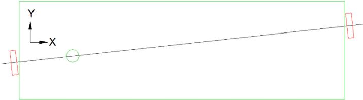
The leadscrew is not parallel to the movement of the table. However, the leadscrew bearings are bolted to the table forcing the leadscrew to follow the ways. The nut (green circle) is bolted to the apron which contains the ways.
