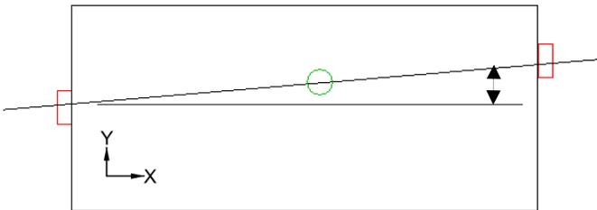
This instrument can tell us when we have zero yaw. When yaw is zero, the leadscrew is parallel to the XZ plane.
