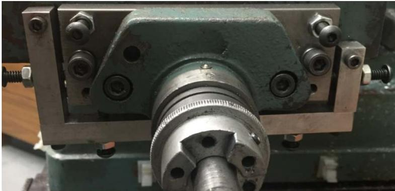
My solution was to make a new surface for the bearing block. This surface can be set at any small angle relative to the end of the table. In order to minimize deflection, the surface is made from 1/2" steel.
