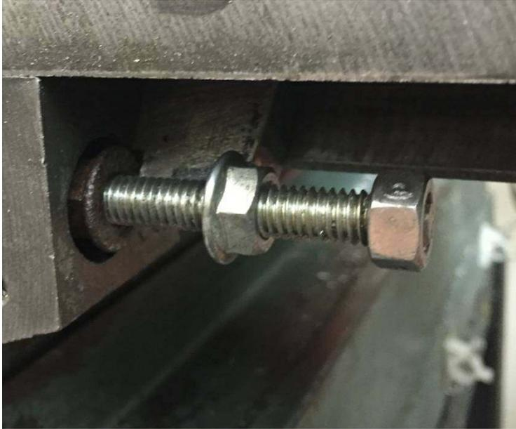
The key action here is to carefully adjust the X gib to be snug but without "excessive" drag and lock its position relative to the apron. See <http://rick.sparber.org/GR.pdf> for details of how I modified the locking mechanism.
