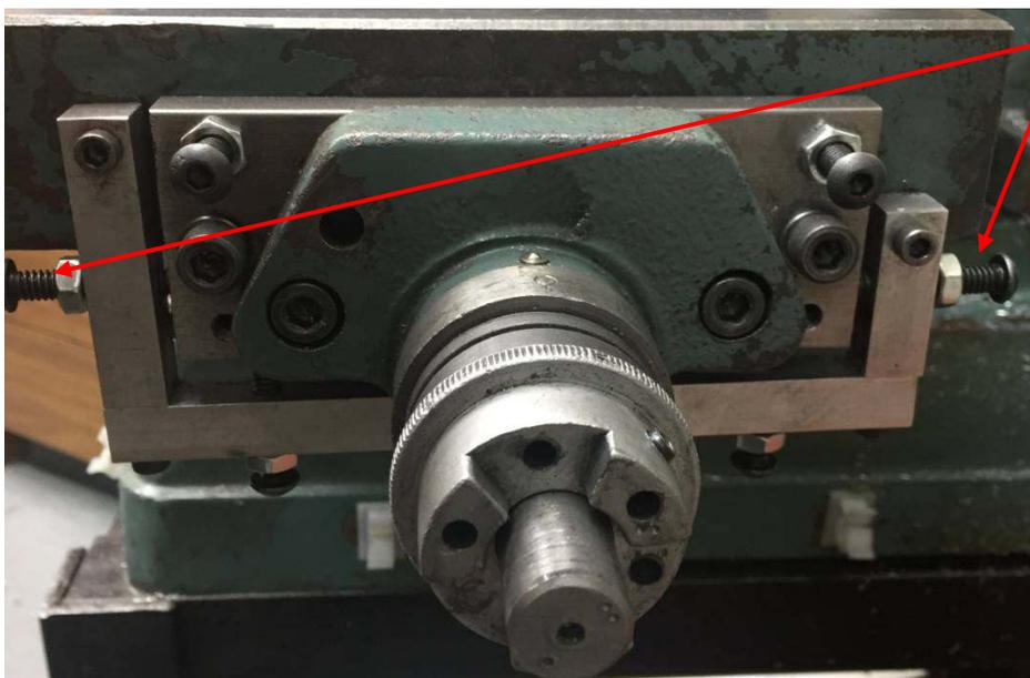
The horizontal jack screws are adjusted until the yaw equals zero. Then the loose horizontal jack screw is tightened to lock this position.
