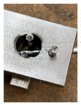
I drilled a hole in the arm that accepts both pins. In this way my arm pivots around two rather than one pin as it resists the bending force. I also flipped the arm over to insure that the wire pushes on the base of each dowels. That minimizes the bending moment.
