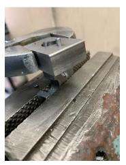
Here you can see how the arm pin clears the base due to the cut out. In the finished design, I'll just use a shorter block for the base.
