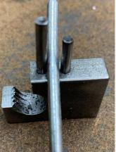
Here you see two dowels spaced a little wider that the diameter of my wire. This leaves no room for the arm that must pivot around one of the pins in order to form the bend. There is a method to my madness.
