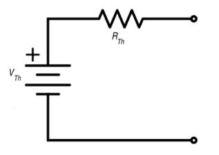
A battery can be modeled by an ideal voltage source,  $V_{Th}$ , and an ideal resistor,  $R_{Th}$ . When no current flows, the voltage measured at the terminals will equal  $V_{Th}$  because there is no voltage drop across  $R_{Th}$ . As the current increases, more voltage is dropped across  $R_{Th}$ , so the measured voltage drops. All of this happens while  $V_{Th}$  remains unchanged.
