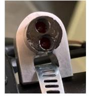
The result is displayed on two red LEDs mounted on my handlebars. This scheme tells me the State Of Charge with a precision of  $\pm 5\%$ . While far from perfect, it is an improvement over measuring voltage.
