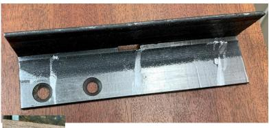
A piece of scrap 1/8" X 1½" X 1½" angle 5" long engages the vise jaws. I chose to drill and tap the angle in three places 10-32, and cut the screws flush after installation.
