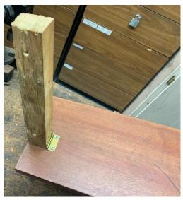
The support leg was cut-to-fit for length. As I install the table in the vise jaws, this leg flops down, read to support the end of the table. It flops back flat when I raise the table for storage.
