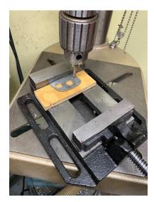
But in this case, my movable jaw cannot reach the stock because my scrap of wood is too wide. Now, I could cut the wood to be narrower but this will also weaken it. I prefer a solution that doesn't require constantly cutting bits of support wood. Besides, I'm always looking for new ways to do old things.
