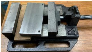
The extension jaw is placed on the vise ways overlapping the wood.
