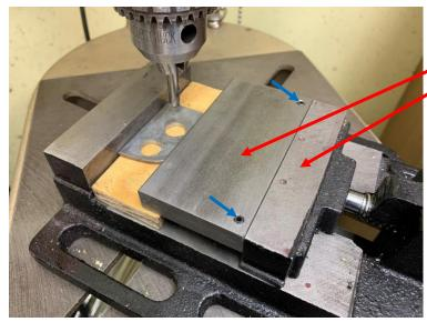
My solution was to make an extension jaw. It extends the movable jaw *over* the wood scrap. And if this wood is replaced by some with a different thickness, two set screws (blue arrows) can be adjusted to return the extension jaw to level.
