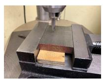
Say I wanted to drill a hole in this piece of stock and not "tag" my drill press vise. It is common practice to place a piece of wood under the stock. The wood must be strong enough to resist the downward force, wide enough to provide stability yet narrow enough to allow the movable jaw to contact the stock. All that is true here.
