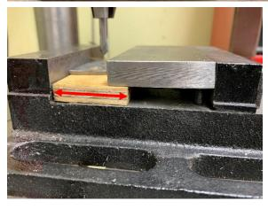
Note that the wood can be almost as wide as the extension jaw and not interfere.
