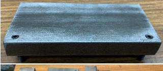
The extension jaw is made from a ½ inch by 2 inch bar of mild steel that runs the width of the movable jaw. I drilled and tapped two holes near the back corners 8-32 and threaded in set screws.
