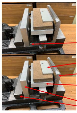
The fixed jaw was trimmed down so it would fit in the vise when fully opened.
