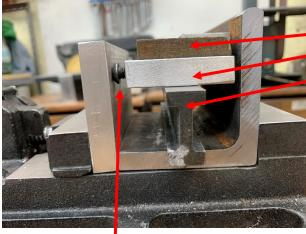
The packing protects the Horizontal jaw and they are supported by a parallel.
