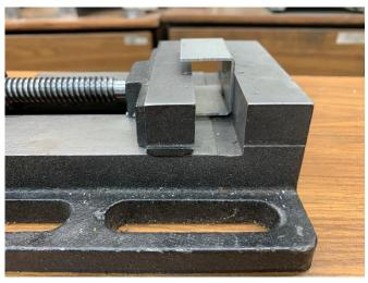
Drilling the outside of a piece of channel can be difficult. The jaws barely clamp one side of the channel, and there is no support for the other side. Typically, the piece jumps out of the vise.
