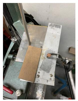
To use my fence, I first make contact between the guide and the front edge of the table. Then I slide it over to the desired distance. And finally, I clamp the fence down.
