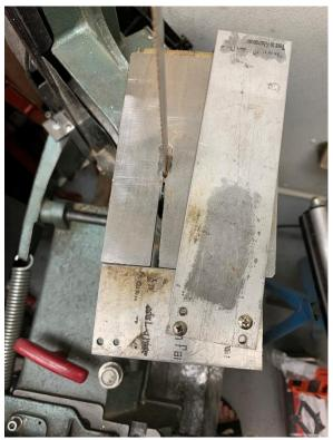
I slapped together a fence using 1/8" X 2" wide strap. It is not square.
