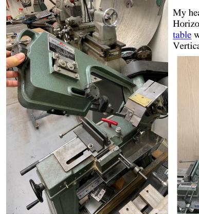
My heavily modified Enco Horizontal/Vertical bandsaw has a <u>flip-down</u> <u>table</u> which I use when the saw is in the Vertical position.
