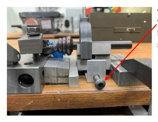
The solution can partially be seen here. Turning the button head screw pivots the V block which changes the altitude of the shaft.
