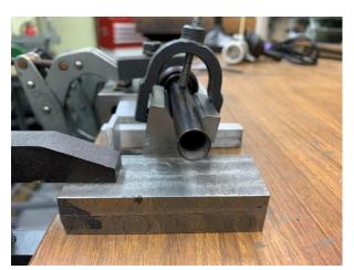
Nothing fancy about the attachment. It is just a scrap of aluminum channel cut down on one side and drilled/tapped on the other.
