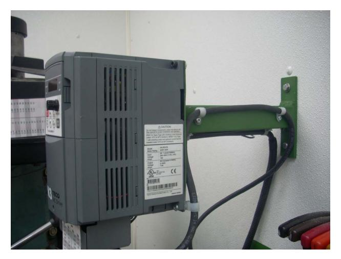
I wanted the VFD to be about 1' closer to me than if it was wall mounted. I also needed it to be away from the wall because the wall is plastic coated and therefore flammable. The user's manual says I must be at least 2" from such surfaces. My solution was to cut 1' of 1.5" square tubing with about a 10° angle on one end. This angle let me locate on a stud yet have the VFD facing me at a comfortable angle.
