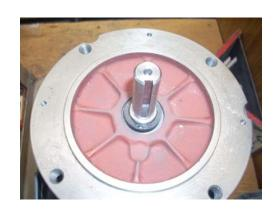
The shaft is 0.625" in diameter and the key slot is 0.125" wide and about 1.5" long.
