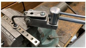
I have many Socket Head Cap Screw fasteners which take an Allen wrench. Sure, I can buy Allen wrenches that accept a standard 3/8-inch drive. But I've already got plenty of bare Allen wrenches. As a proof of concept, here is an Allen wrench bolted to my adapter. Distance 2 must be measured to get the correction factor.
