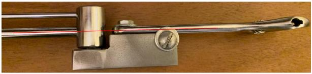
This side view shows how the adjustable wrench is aligned with the bar (red line).
