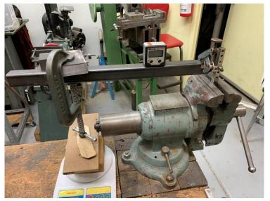
I selected a heavy steel piece of square tubing. At the left end I clamped a chunk of steel. The end of the C-clamp rests on a pile of wood<sup>3</sup> supported by a digital scale.
