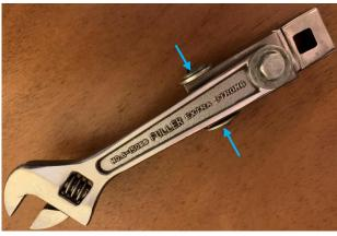
The washers on the flanks of the attachment (blue arrows) limit the wrench's side to side motion. If this small pivoting causes a reduction in accuracy, I will make blocks to replace the washers that are snug against the wrench.
