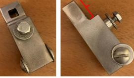
Here is my attachment. It was cut from a bar of 1-inch by 1-inch mild steel about 3-inches long.
