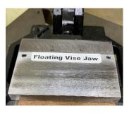
Using toner transfer, those labels can look as professional as what comes out of your laser printer plus will be far more durable. Here we have toner transferred onto powder coated aluminum which has been glued onto the surface of the tool.
