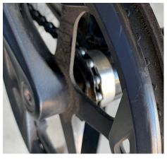
The chain comes to rest on the crank box. Yes, that area does get a little greasy, but it won't get on you. At this point, the cranks freely turn, so it can't jam into the frame and lock up the rear wheel.
