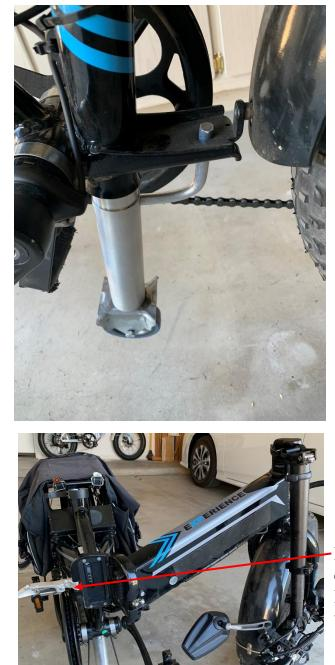
The rod has just enough spring to slide through the existing hole in the rear fender support and lock into place.
