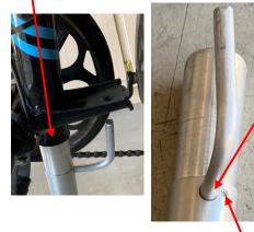
Then I cross-drilled a 3/8 inch hole just below the transition to full diameter.
