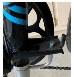
I loosened the setscrew. With the cylinder in the down tube, I adjusted the bent rod so it would enter the fender support plate with a slight flexure. This force was enough to retain the assembly until I lowered the bike onto the wheel.
