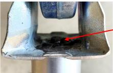
I found a bit of scrap steel that was a close fit to the axial hole in the leg. On the end of the scrap was a 3/8 inch spigot, <sup>1</sup>/<sub>4</sub> inch tall which became my mounting post. With the wheel frame upright and supported on a firebrick, I fluxed the mating surfaces and then pushed the pieces together. Using a MAPP torch and some silver braze, I formed the joint. The
