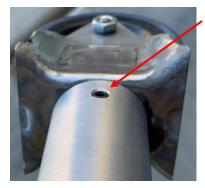
Next, I drilled and tapped a <sup>1</sup>/<sub>4</sub>-20 hole near the bottom of the leg. The installed setscrew locked the mounting post after I had roughly aligned the wheel to the major axis of the bike.
