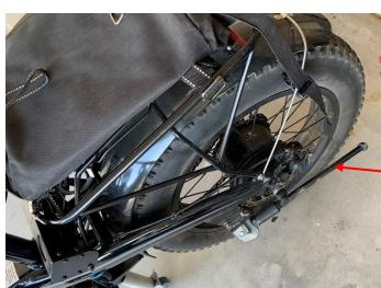
The attachment secures the front wheel to the back wheel while permitting both wheels to turn. I don't need much strength here, just enough to prevent the front wheel from going out on its own.
