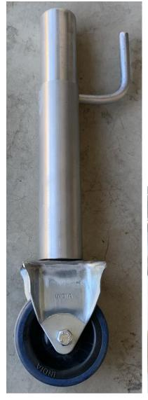
The removable third wheel consists of a fixed wheel secured to the bottom of a thick aluminum rod. An arm extends out the back, which engages with a hole in the bike's frame to prevent the assembly from pivoting.
