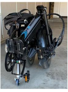
Since the crank is not connected to the chain, I can now smoothly roll the folded bike forward and backward.
