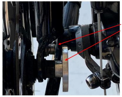
Looking down between the wheels with the bike folded, you can see the kickstand engages <u>the disk</u> from below, holding the wheels together.
