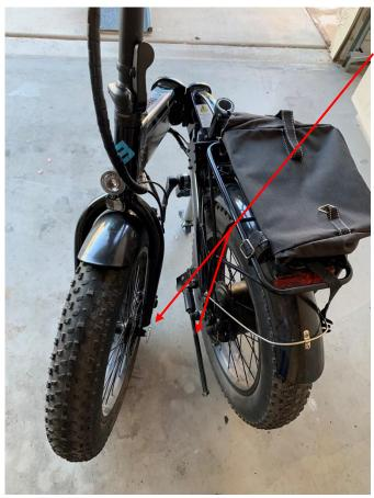
I swing the front wheel until the axle disk contacts the kickstand. Momentarily pushing down on the kickstand, it catches the disk.
