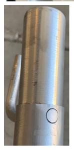
After tightening the setscrew again, I trimmed off the excess rod, so it was flush with the cylinder.
