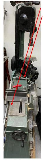
Is this machined surface on my  $4 \ge 6$  bandsaw parallel to my pivot shaft<sup>2</sup>? This is not a wildly dreamt up question. I needed to know in order to improve the cutting accuracy of my saw.
