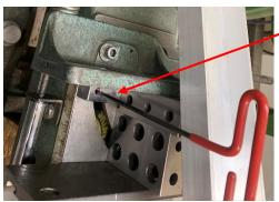
I built a sine bar and put my 1-2-3 block on top. While pushing on the channel,
