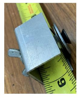
To install, I first slip the tap under the washer so it rests inside the U-shaped piece of aluminum.
