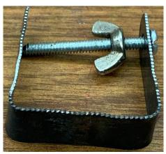
Locate an end of the hacksaw blade with a hole in it. Use the torch to heat up the blade about 1 inch from the end.
