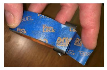
To cut, stick the tape back on the face of the blade, tilt it so the teeth point up, and pull the tape along the teeth.
