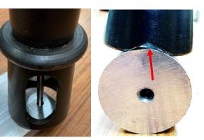
The outer support sets the tap chuck perpendicular to a flat or round surface.
