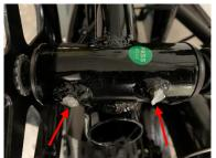
As far as I could see, all of the damaged bikes had the bottom bracket support leg broken off. It was aluminum and sheared just beyond the weldment.
