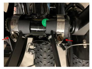
A pair of stainless steel hose clamps securely locks the assembly to the bottom bracket.
