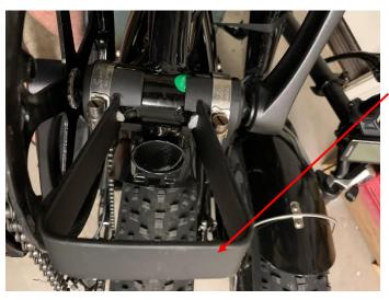
I still must cover the bottom of the support leg in thick rubber. That paint will scratch off the first time it rests on concrete and is slid around.
