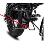
The second bike we looked at had zero miles on it. I was out the door for \$835, which includes \$63 in tax. This support leg is needed when the bike is folded up. It keeps weight off of the front sprocket.
