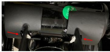
I estimated the size of the two cut-outs and then sawed and filed until it fit<sup>2</sup>. I had to file a bevel on the inside of the curve to clear the weldments. This close fit prevents the support from rotating.
