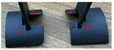
I am a little concerned about my method of attaching the base to the support leg. Due to bad planning, I didn't leave much metal for the joints. I was concerned that welding would burn through. So, instead, I silver brazed the joint. Because brazing fills the gaps and forms a fillet, it is strong. The part that broke off the bottom bracket was aluminum, and I'm using steel.
