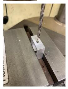
I drilled a through-hole with a #27 drill.
