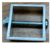
After deburring plus rounding all edges, I ran a 6-32 bolt through the hole and secured it with a locking nut. Then I sawed off the excess bolt and filed it smooth.
