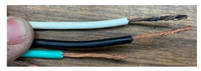
Using the black wire as a guide, I cut and stripped the white wire to match.
