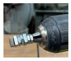
When the rod is full of tested nuts, I hold the group and reverse the drill. This spins them all into my hand.
