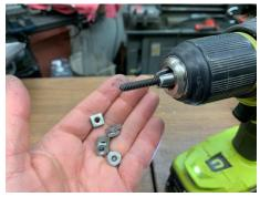
I pick up a handful of nuts and place them, one at a time, against the end of the *slowly* turning rod. If it freely engages, I run the nut all the way in. If it catches, I manually turn the nut backwards about ½ turn and place it aside.
