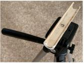
In the center is a hole drilled and tapped \(^1\lambda\) - 20. Mine is not centered radially so the open end of the U faces a little forward. No matter, it still works.
