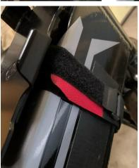
Next, I install a second strap to be doubly sure the carrier will not fall off or twist.
