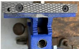
After mounting the jaw plate, I used the hole as a guide with the #7 drill mounted in my hand drill. Then I opened out the jaw plate's hole with a F drill (0.257 inches in diameter). This insures that the F drill hole is perfectly aligned with the #7 hole.
