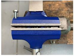
One solution is to add a jack screw at one end of the vise. Since I'm right handed, I put the jack screw on the left end.
