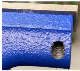
I then passed my ½-20 tap through the jaw plate and cut threads in the casting behind it. Note that the threads broke out the back side. Going in from this back side with the tap would have been near impossible.
