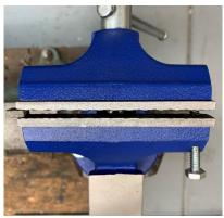
The threaded hole is usable but did not come out as perpendicular to the jaw face as desired. I should have used my
