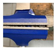
Clamping small parts in a light weight vise can be less than satisfactory. The movable jaw tend to tilt providing uneven clamping force.
