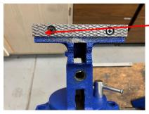
I started by removing the movable jaw assembly. Then I marked the location of the hole to be drilled in the fixed jaw plate.
